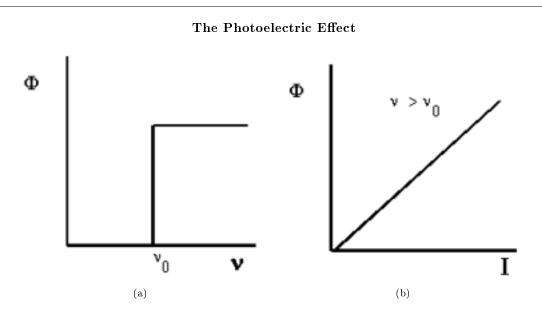
**Figure 5.1:**  $\Phi$  is the photoelectric current,  $\nu$  is the frequency of incident light, and *I* is the intensity of incident light. (a) For photoelectrons to be emitted, the light frequency must be greater than a threshold value. (b) If the frequency is high enough, the number of photoelectrons increases directly with the light intensity.
