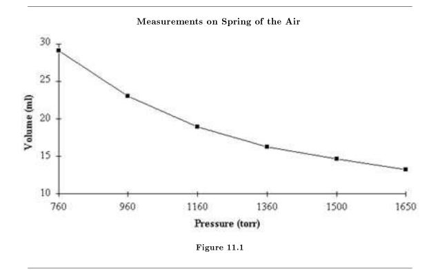
An initial question is whether there is a quantitative relationship between the pressure measurements and the volume measurements. To explore this possibility, we try to plot the data in such a way that both quantities increase together. This can be accomplished by plotting the pressure versus the inverse of the volume, rather than versus the volume. The data are given in Table 11.2: Analysis of Sample Data and plotted here (Figure 11.2: Analysis of Measurements on Spring of the Air).
