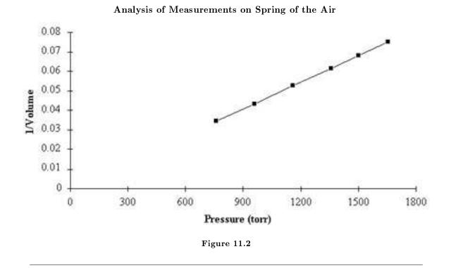
Notice also that, with elegant simplicity, the data points form a straight line. Furthermore, the straight line seems to connect to the origin  $\{0, 0\}$ . This means that the pressure must simply be a constant multiplied by  $\frac{1}{V}$ :
