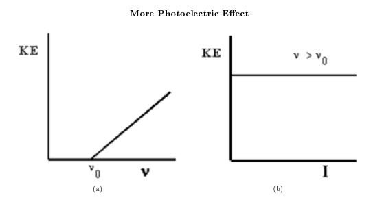
**Figure 5.2:** KE is the photoelectron kinetic energy,  $\nu$  is the frequency of incident light, and I is the intensity of incident light. (a) If the frequency is high enough, the energy of the electrons increases directly with the frequency. (b) However, the energy of the photoelctrons does not depend on the light intensity.
